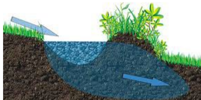
Figure 9 Swale with water infiltrating into the soil. (Stross 2022)
